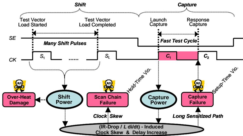
Figure 1. Impact of Test Power in LOC-Based At-Speed Scan Testing
